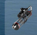
Water Sampler (500ml)
